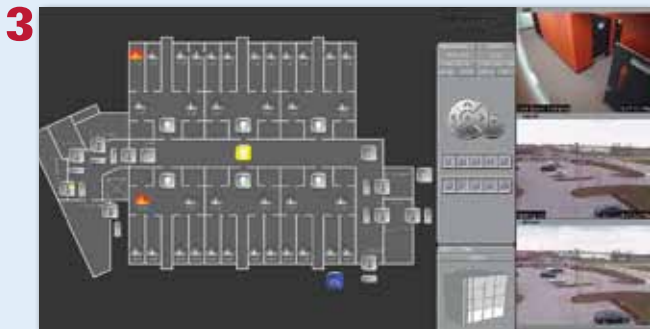
3 Stanley CSS' Corporate Commander PSIM sits atop Conseco Fieldhouse's security and facility management subsystems to facilitate a single point of command and control.
